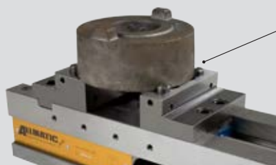
clamping unmachined parts round
