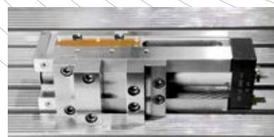
Vice in lateral clamping position
