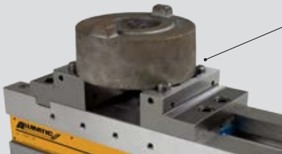
clamping unmachined parts round
