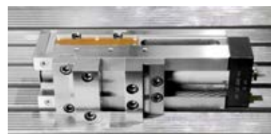
Vice in lateral clamping position
